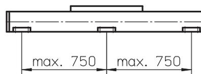
A mounting clamp must be installed at least at every 750 mm to be able to operate the maximum load. Less clamps may be required if less load is being operated, see the additional technical data for more information.
