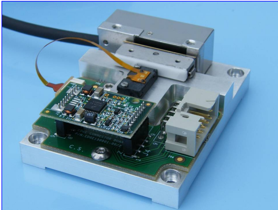
Figure 4: Example of stage based on EDGE motor including ASIC EDGE driver and position encoder (EDGE MOTOR EVALUATION KIT stage).
